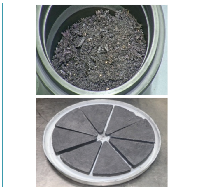
Fig. 2: Uranium dendrites and consolidated ingot
