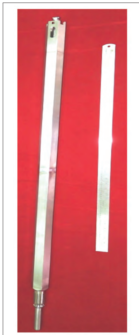
Fig. 4: The special sub-assembly loaded with irradiation capsule
