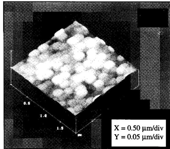
Fig. 3 : AFM micrograph of  $\text{FeNbO}_4$  film
