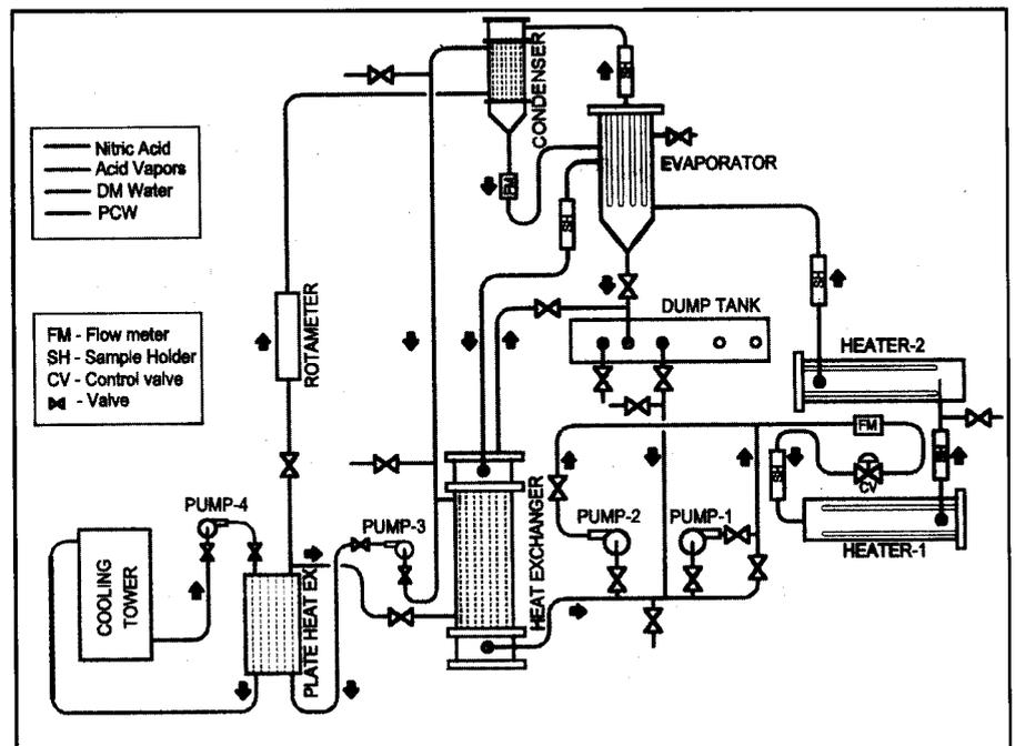
Fig. 1 : Schematic flow diagram of the nitric acid loop
