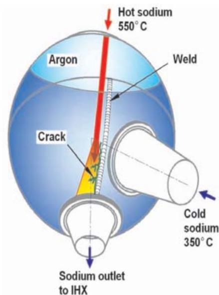
Fig.2: TS in Phoenix expansion tank
