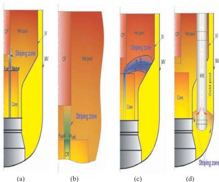
Fig.4: Critical locations where thermal striping occurs in the hot and cold pools of FBR
