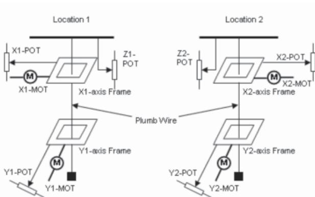
Fig. 3: Diagram of Reactor Vessel Displacement Measuring Device
