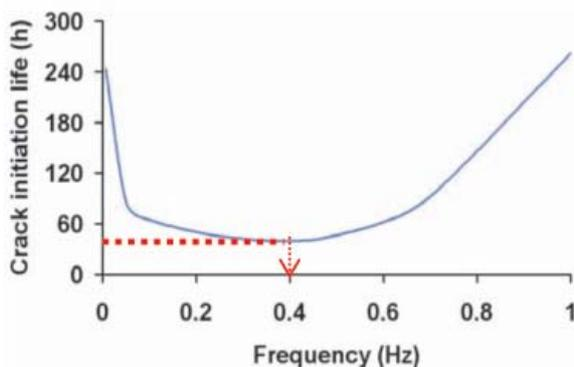
Fig.6: Concept of critical frequency
