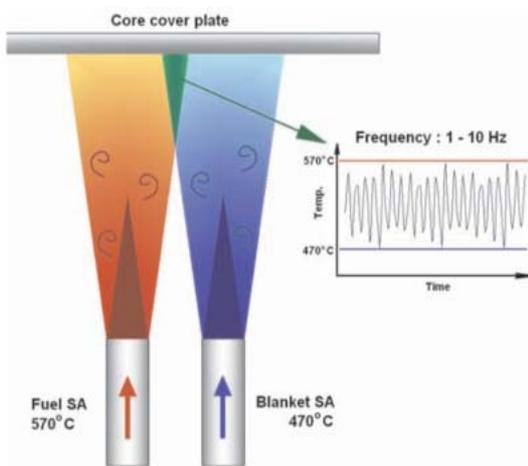
Fig.1: Thermal striping phenomenon
