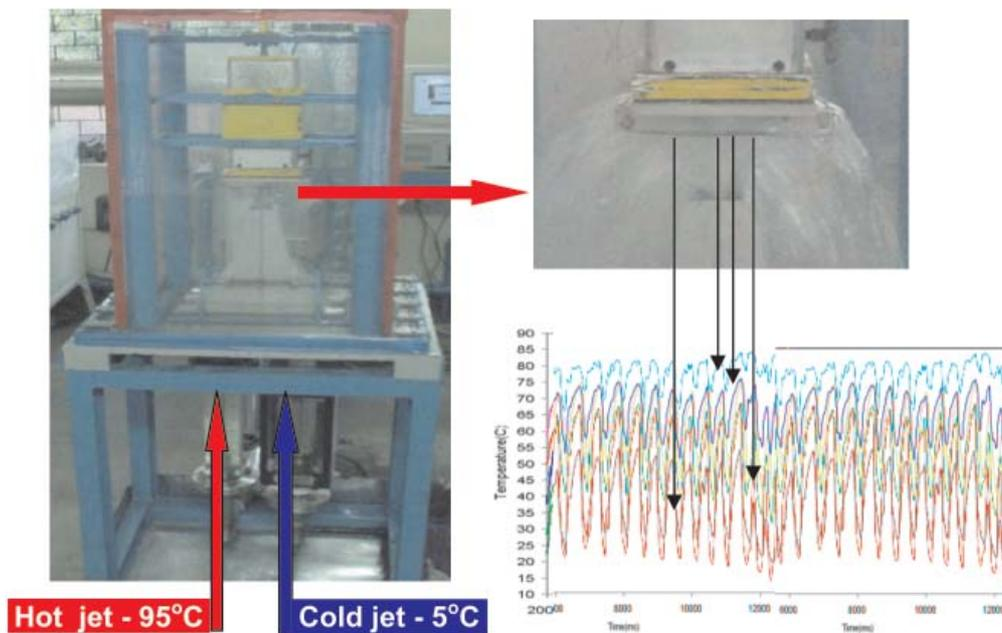
Fig.9 Simulation of thermal stripping with water jets
