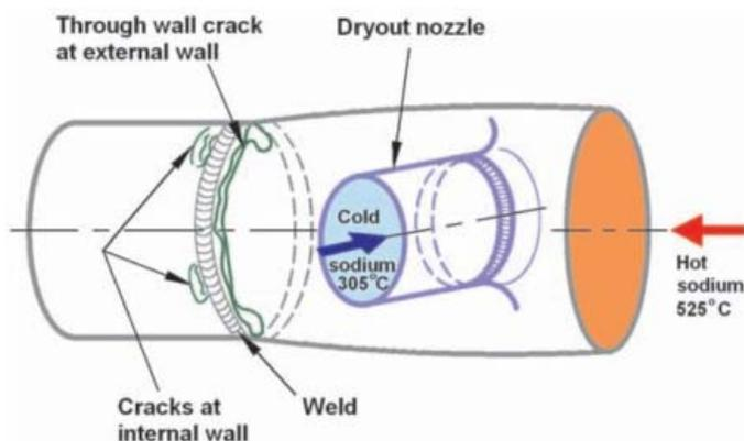
Fig.3: TS in SPX-1 Mixing Tee
