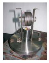
Fig. 4 : A prototype on-line transformer oil monitoring probe.
