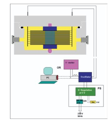
Fig. 1 : Schematic representation of the oil monitoring device.
