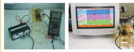
Fig. 2 : a) A typical pulsating sensor based transformer oil field monitoring kit. b) A PC based data acquisition system for the oil monitoring device.
