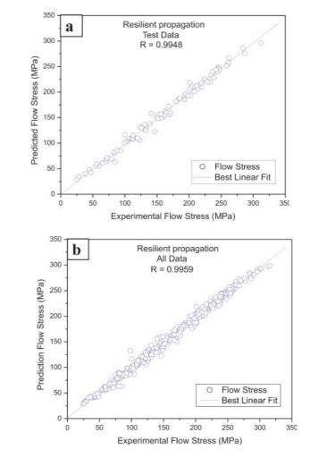
Fig.2: Performance of the network to predict the constitutive behavior of 304L under hot torsion (a) training data set (b) all data set
