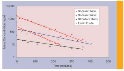
Fig.3 The depletion of mass concentration of sodium compound aerosol along with Fe\_O\_{\_3} and SrO\_{\_3} aerosols
