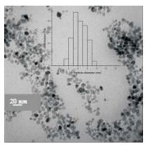
Fig 1. The TEM image of magnetite nanoparticles and the size distribution (inset).
