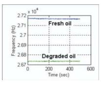
Fig. 3 : Pulse frequencies recorded as a function of time for fresh oil and a sample of service oil.
