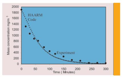
Fig.4: Depletion of suspended sodium compound aerosol mass concentration with time in the absence of gamma field
