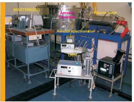
Fig.1 Photograph of Aerosol Test Facility showing plasma torch, aerosol chamber and aerosol diagnostic equipments.
