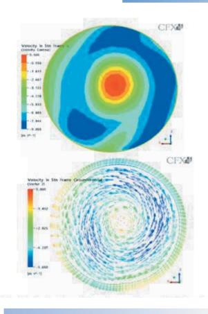
**Fig.3**Axial (top) & Circumferential (Bottom) Velocity
