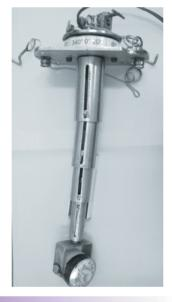
**Fig.1 (b)** 2-Axis Telescopic Scanner (Expanded State)
