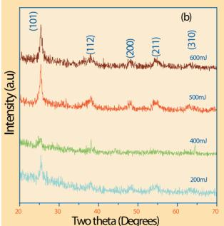
**Fig. 1**GIXRD Patterns of Thin Films Prepared at 673 K in the Laser Energy Range 200 - 600 mJ/pulse at (a) base pressure of  $3.7 \times 10^{-5}$  mbar, and (b) 0.1 mbar  $O_2$  partial pressure.
