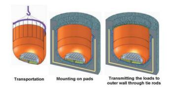
**Fig.3**Erection of Main Vessel Along with
