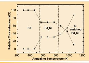
**Fig.2**Auger Electron Spectroscopy Results in terms of Relative Concentration of Pd (solid circles) and Si (open circles) as a Function of Annealing temperature for Pd/Si System. The Temperature Regions Corresponding to the Transformation of the over-layer from Pd to Pd $_2$ Si and Si-enrichment of Silicide are indicated by vertical dotted lines.
