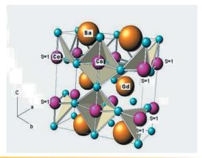
**Fig. 1 (a)**The Crystal Structure of Ideal GdBaCo<sub>2</sub>O<sub>5.5</sub> Gd, Ba and Co are marked, the atoms marked blue are oxygen.
