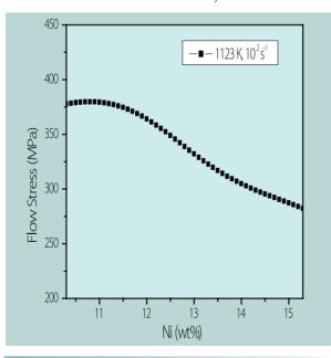
**Fig. 1**Neural Network Predictions for the Influence of Ni on Flow Stress of AISI Type 304 Steel at 0.5 Strain Level
