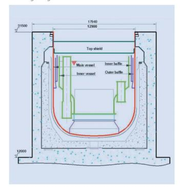
**Fig.1**Schematic Sketch of Reactor Assembly Vessels
