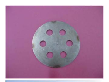
**Fig. 1 a**Typical 4-plate Orifice Plate (zone-10)
