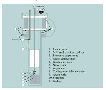
**Fig.1**Schematic of Electrowinning Setup
