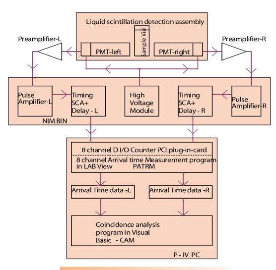
**Fig.1**Liquid Scintillation Coincidence Counting System
