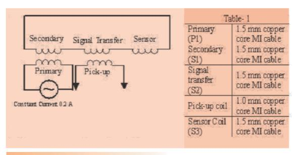
**Fig. 1**Circuit Diagram of Prototype ECPS
