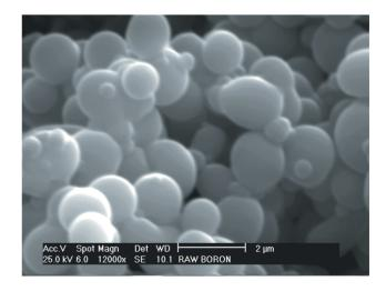
**Fig.2 (b)**SEM Image of Processed Boron
