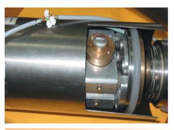
**Fig.2**Sensor Inserted inside a Mock-up Tube
