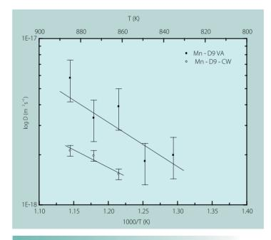
**Fig.4**Bulk Diffusion of <sup>54</sup> Mn in Alloy D9 in Annealed and Cold Worked Conditions
