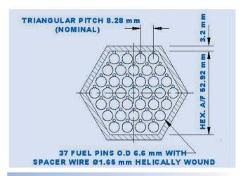
**Fig.2**Cross-section of 37- pin Sub-assembly
