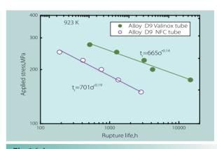
**Fig. 1 (a)**Relationship Between Applied Stress and Rupture Life of Valinox and NFC Tubes at 923 K.
