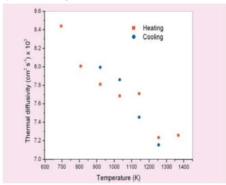
**Fig.2**Variation of Thermal Diffusivity as a Function of Temperature
