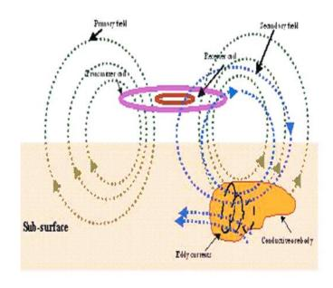
**Fig. 1**Principle of Time Domain Electromagnetic Method
