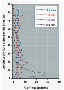
**Fig.3**Debris Distribution In 5ppm Concentration Runs
