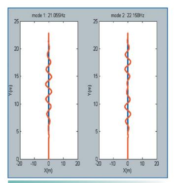
**Fig.2**First two Mode Shapes of SG Tube
