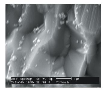
**Fig. 1**Scanning Electron Micrographs of YDT Pellet Samples Sintered at 1923 K: a) Surface Morphology and b) Cross Sectional View
