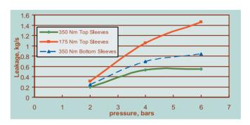
**Fig.4**Total leakage though sleeves nut
