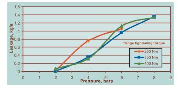
**Fig.2**Leakage Through the Top Flanges,
