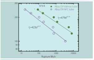
**Fig. 1 (b)**Relationship between Applied Stress and Rupture
