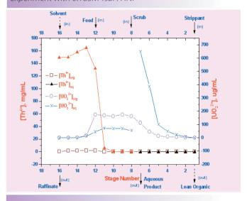
**Fig.4**Stage Profiles for the Separation of U (VI)
