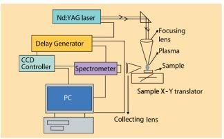
**Fig.1**Experimental Set up of the Laser
