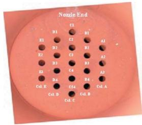
**Fig. 1**Tube Sheet Layout of the SGTF with Tube Numbering
