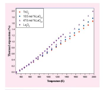
**Fig.2**Thermal Expansion (%) as the Function of Temperature for ThO<sub>2</sub>-LaO<sub>1.5</sub> Solid Solutions
