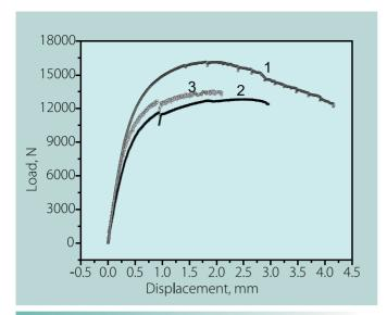
**Fig. 1**Plots of Load (P) versus Load Line Displacement (LLD) for the Ramp tests. (In all cases, sudden load drops corresponding to pop-in crack extensions are observed.)
