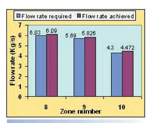
**Fig.2 b**Comparison of Required and Achieved Flow at Rated Pressure Drop.
