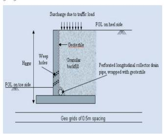
**Fig.1.** Typical Cross Section of Retaining Wall
