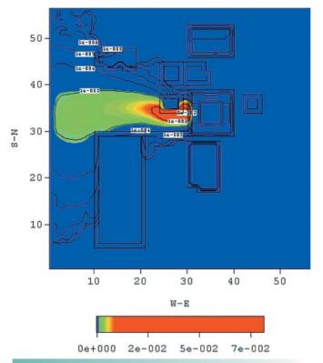
**Fig. 3**Plume Dispersion and Contours for 1 m/s Wind Impinging on the Western Face of the PRBR Complex.
