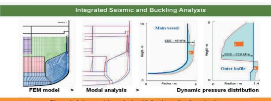
Phase-1: Axisymmetric analysis with fourier option for seismic response
