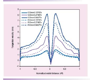
**Fig.3**Tangential Velocity Profiles for 125 & 150mm Diode for Three Inlet Velocities
