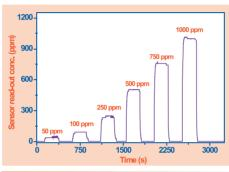
**Fig.3**Sensor Readout for Set Conc. of Hydrogen
