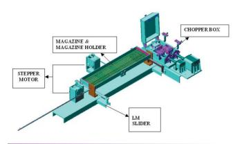
**Fig. 1**Schematic of Chopper for FBTR Fuel.
