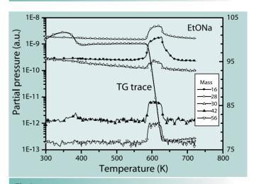
**Fig.3**Typical TGA-MS Curve for Decomposition of Sodium Ethoxide at a Heating Rate of 5 K min<sup>-1</sup>
