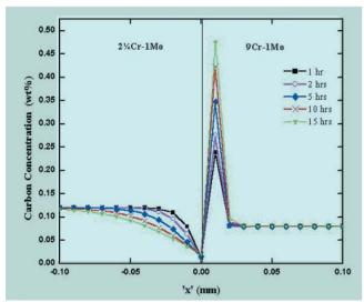
**Fig. 1**Simulated Carbon Concentration Profiles
