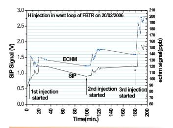
**Fig. 2**Response of Electrochemical Hydrogen Meter to Hydrogen Injections in FBTR
