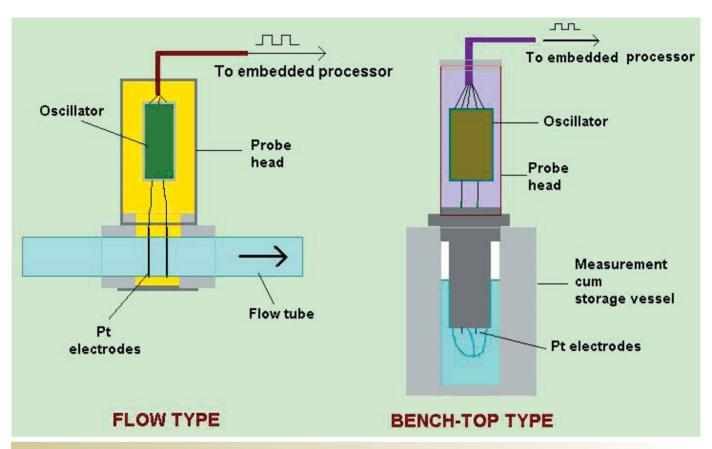
**Fig.1**Schematic Representation of Flow and Bench-top Type Conductivity Probes.
