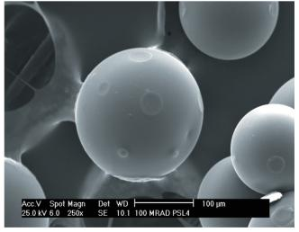
**Fig.2**Scanning Electron Micrographs of Unirradiated and 100 MRad Irradiated Tulsion A-PSL 4.
