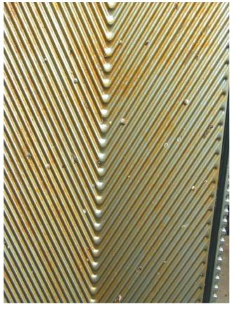
**Fig.6**A View of Barnacle Settlement on PHE
