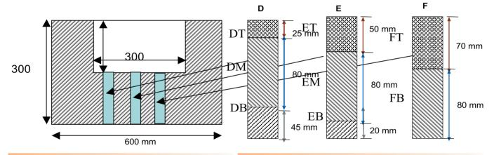
**Fig. 1 b**Schematic of the Cross Section of the Concrete Blocks
