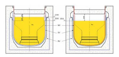
**Fig.2**Sodium Levels under Normal and Main Vessel Leaked Conditions
