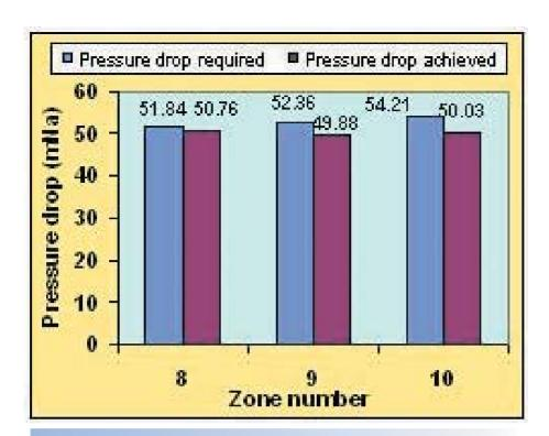
**Fig.2 a**Comparison of Required and Achieved Pressure Drop at Rated Flow Condition.
