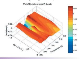
**Fig. 1**A Pictorial Representation of the Error Surface for Prediction of Aqueous Density of AHA Solutions at Several Concentration and Temperature Levels
