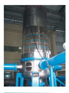
**Fig.1** 5/8 Scale Model Surge Tank
