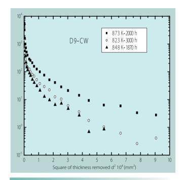
**Fig.3**Residual Activity of  $^{54}$ Mn as a Function of  $d^2$  in CW Specimens
