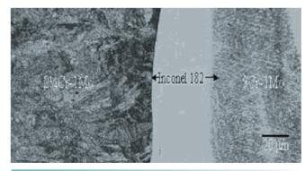
**Fig.3**Optical Micrograph Showing the Absence of Hard and Soft Zones in Dissimilar Weldments of Ferritic Steels with Inconel Interlayer After PWHT at 1023 K for 1h.
