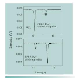
**Fig.2**Typical Mass Spectrum of Isotope of B Obtained for  $B_4$ C Pellets.
