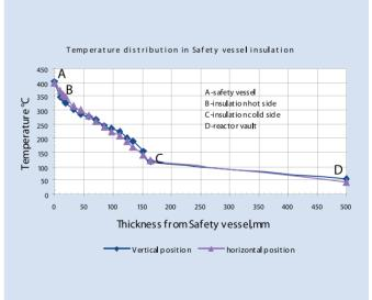
**Fig.2**Temperature Distribution in Safety Vessel Insulation
