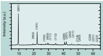
**Fig.2**X-Ray Diffraction Pattern of Sodium Ethoxide
