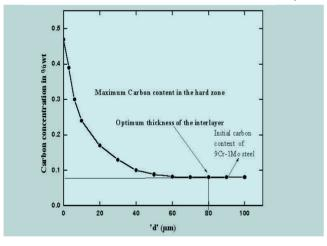
**Fig.2**Variation of Maximum Carbon Content in the Hard Zone with Increase in the Thickness 'd' of the Interlayer.
