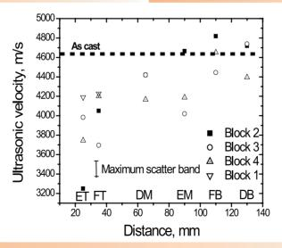
**Fig. 2**Variation in Ultrasonic Velocity with Average Distance from Centre of Core Specimen to the Surface Exposed to Sodium Fire for the Four Blocks (ET, FT, DM, EM, FB) and DB indicate the Core Specimens Extracted from Different Depths, as shown in Fig. 1b.
