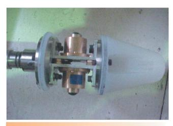
**Fig. 1 Eddy Current Sensor with Head Assembly**
