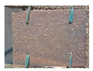
**Fig.4**Fouling on a Week old Panel Exposed During
