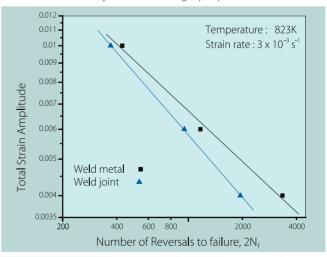
**Fig.2**Comparison of Low Cycle Fatigue Resistance of Weld Metal and Weld Joint at 823 K.
