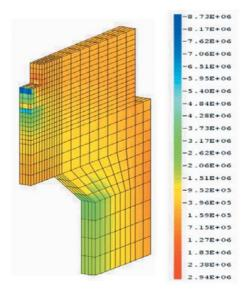
**Fig.4**Axial Stress In the Upper Lateral Region Under Net Load
