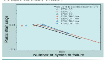
**Fig.3**Coffin - Manson Plot showing Strain-Life Relation at Three Temperatures.
