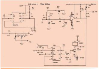
**Fig. 2**Bubble Detector Based Criticality Incident Detection and Alarm System
