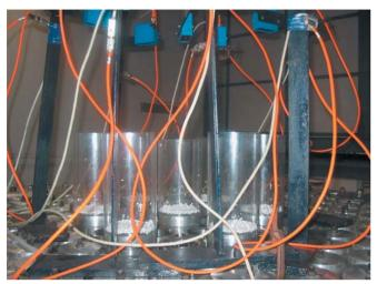
**Fig.3**Laser level probes arrangement for leakage though top sleeves nuts
