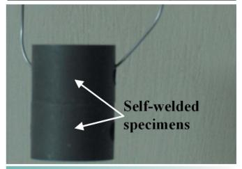
**rig. I** Cold Worked Alloy D9 Specimens in Self-welded Condition
