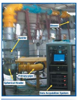
**Fig.4**Experimental Test Facility for Hydraulic Testing of Spherical Header established at FCRI, Palghat
