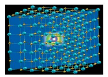
**Fig.3**Computed Positron Density Profile along (110) Plane in the Completely Relaxed TiC supercell with C Vacancy at the Body Centre. The colour grading from blue to white is representing the increasing positron density.
