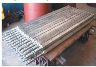
**Fig.1**Fabricated Dummy Fuel Sub-assemblies
