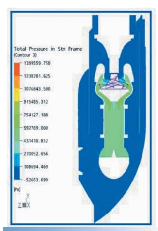
**Fig.2**Pressure distribution in a Section through the Pump
