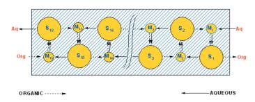
**Fig.2**Counter-current Flow of Organic and Aqueous phases in a Mixer-settler
