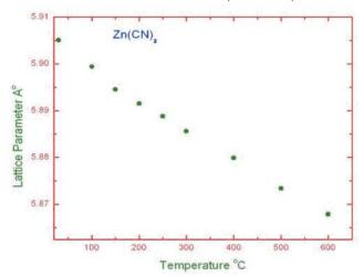
**Fig.2**Lattice Parameter Vs Temperature Showing Lattice
