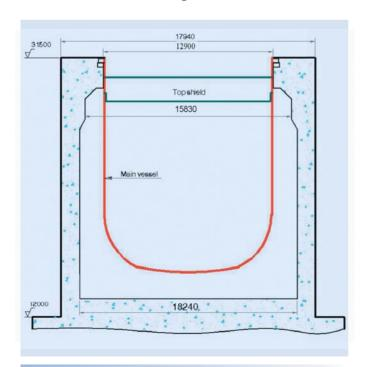
**Fig.1**Reactor Vault Outer Wall Supporting the Main Vessel
