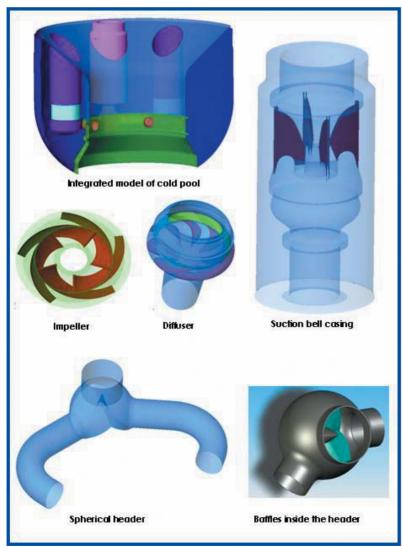
**Fig.1**Integrated CFD Model of Cold Pool
