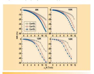
**Fig.3**The MR Defined as (R(0)-R(H))/(R(0)) in Percentage, Shown for Different amounts of Ce Substituted at the Gd site in GdBaCo<sub>2</sub>O<sub>5.5</sub>, Compared at Various Temperatures.
