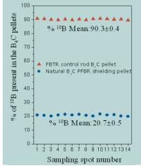
**Fig.3**% of <sup>10</sup>B Measured over 40mm dia  $B_4$ C pellet along a Straight Line: Laser spot dia: ≈ 400 $\mu$ m
