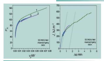
**Fig. 3**(a) Plots of  $v_p$ - $P_N$  Corrected for Crack Extension from Normalization Method Modified with Small Pop-in Assumption. (b) Single specimen J-R curves obtained using normalization method with "small" pop-in assumption for all the four tests.
