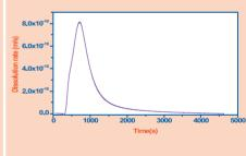
**Fig.7**Dissolution Rate of Depleted Surface of Sodium-exposed SS 316LN
