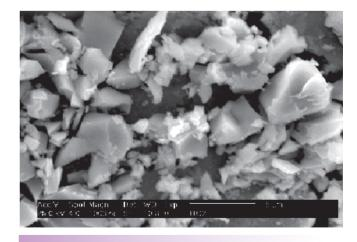
Fig. 1 SEM Micrographs of  $UO_2$  Deposit Obtained by Controlled Potential Electrolysis of 40 mM Solution of Uranyl Nitrate in bmimCl on a Pt plate (1cmx 1 cm) at -0.8V for 18-20 hrs.
