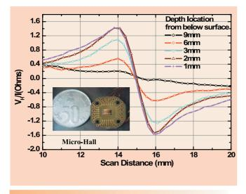
**Fig.2**Typical Voltage Signal (tangential component of magnetic field) of Micro-Hall Sensor for Sub-surface Notches at Different Depth Location in Carbon Steel Plate.
