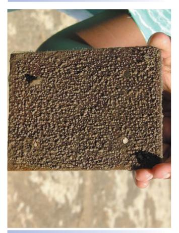
**Fig.3**Fouling on a Week old Panel Exposed During May (18.05.06-25.05.06)
