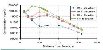
**Fig. 2**Aerosol Dispersion in Open Terrain for 1 m/s Stable Wind
