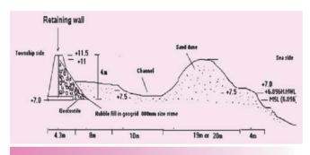
**Fig. 1**Cross Section of Tsunami Protection Wall
