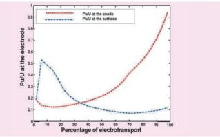
**Fig.2** Variation of Ratio of Pu/U at the Liquid Cadmium Anode and Liquid Cadmium Cathode
