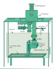
**Fig. 1**Home-built Reflectron Time-of-Flight Mass
