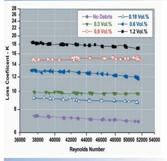
**Fig.5**Variation of Pressure Loss Coefficient with Reynolds Number (for 1.6mm)
