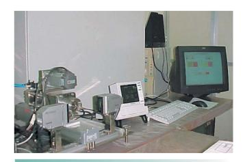
**Fig. 1**Remotely Operable Optical Micrometer System
