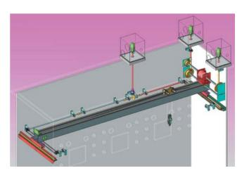
**Fig.1** Schematic of a Special Mini Crane for Hot Cell Application.
