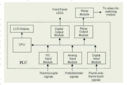
**Fig.3**DMD Controller Block Diagram
