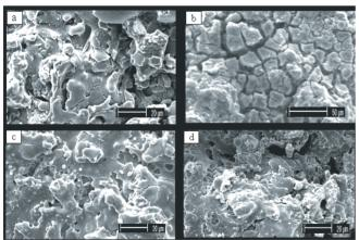
**Fig. 1**SEM Micrographs of Partially Stabilized Zirconia Coated over type 316L SS in (a) as-coated, (b) 5 h exposed, (c) 100 h exposed, and (d) 500 h exposed to molten LiCl–KCl salt
