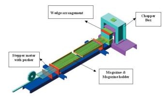
**Fig.2**Schematic of Chopper for PFBR Fuel.
