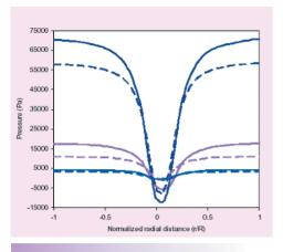
**Fig.6**Radial Pressure Distribution for 125 & 150mm mm Diode - Three Inlet Velocities
