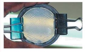
**Fig.3**CE Gel Formed in the Quartz Cell
