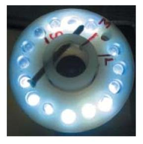
**Fig.2** CCD Camera with LED Lighting
