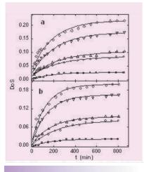
**Fig.1**Degree of Swelling (DoS) a) 0.5% and b) 1% MBA gels.  $\Box$  - 0.1N, O-0.5N,  $\Delta$ 1N,  $\nabla$ -2N & ◊ - 3NHNO<sub>3</sub>
