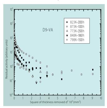
**Fig.2**Residual Activity of <sup>54</sup>Mn as a Function of d<sup>2</sup> in VA Specimens
