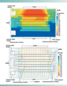
**Fig.2.**Velocity and Temperature Profiles in the Recommended Design of AHX
