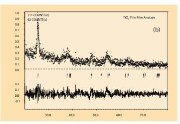
**Fig.2**A Typical XRD Pattern of Results of Rietveld Analysis of (a) Rutile thin film, and (b) Anatase thin film data. The position of Bragg Reflections are indicated by vertical bars. The solid line and the dotted line represent calculated and observed intensity, respectively. The lower part of the diagram (horizontal line) shows the deviation between the experimental and the calculated intensities from the refined model.
