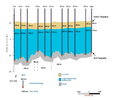
**Fig.2**Depth-Section along Traverse-1 (Ch.0-360m) at FRFCF Site, Kalpakkam
