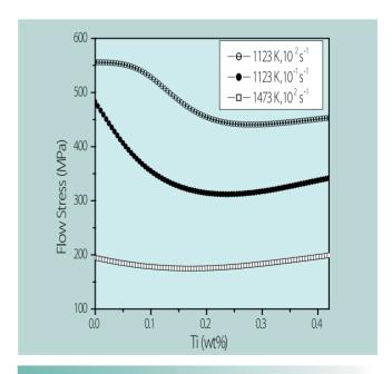
**Fig.2**Neural Network Predictions for the Influence of Ti on Flow Stress of D9 at 0.5 Strain Level
