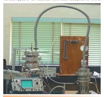
**Fig.1** *Ion Source for Intense Pulse Neutron Source*
