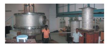
**Fig. 1**Experimental Setup of Grid Plate Leakage
