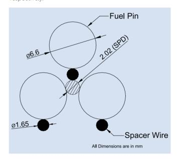
**Fig.4**SPD: Sub-channel Passage Diameter
