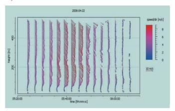
**Fig.3**The Wind Velocity Profile over the Sea from Sodar as a Function of Height and Time
