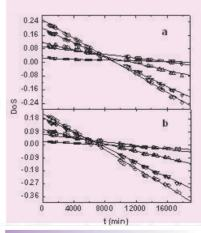
**Fig.2**Degree of Swelling (DoS) at Longer Times.  $\square$  - 0.1N, O-0.5N,  $\triangle$ 1N,  $\triangledown$  -2N &  $\lozenge$  - 3NHNO<sub>3</sub>
