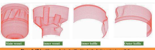
Phase-2: 3D buckling analysis at critical instants during seismic excitations
