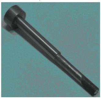
**Fig. 1**Photograph of as-brazed Joint of IN600
