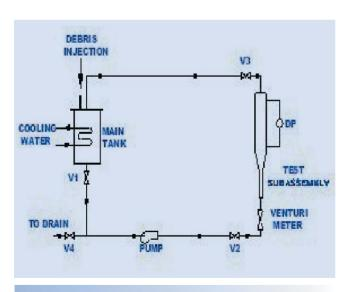
**Fig.1**Schematic Layout of Experimental Loop
