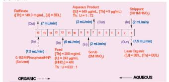
**Fig.3**Flow Sheet for the Integral U/Th Separation Experiment with 0.183M TsBP/HNP
