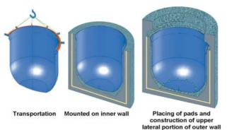
**Fig.2**Safety Vessel Erection
