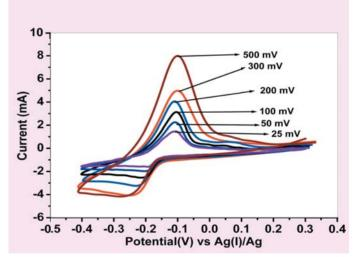
**Fig.2**The Cyclic Voltammograms for a Glassy Carbon Electrode in MgCl<sub>2</sub>-NaCl-KCl Eutectic Melt containing 9.47 x 10<sup>-6</sup> mol cm<sup>-3</sup> LaOCl at 873 K. Apparent Electrode area: 0.346 cm<sup>2</sup>
