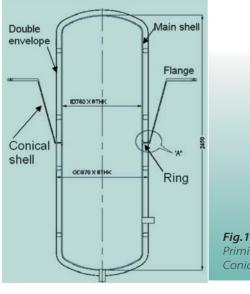
**Fig. 1**Priming Tank with Conical Support
