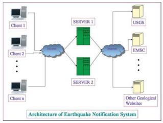
**Fig. 1**Operation Schematic of Earthquake Notification System
