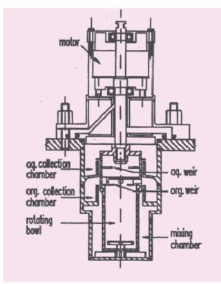
**Fig.1**Schematic of a Centrifugal Extractor Stage
