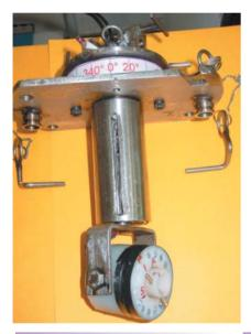
**Fig.1 (a)**2-Axis Telescopic Scanner (Collapsed State)
