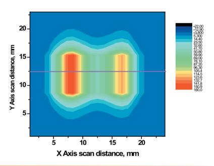
**Fig.4**The image of Sub-surface Defect (EDM notch, 5 mm below surface) in a 6 mm thick Stainless Steel plate, Generated by the Integrated EC-GMR Probe
