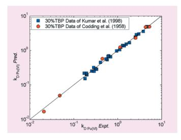
**Fig.2**Parity Plot for Pu(VI) Distribution Coefficients in PUREX Process.
