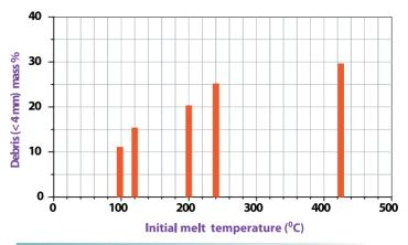
**Fig.3**Effect of Melt Temperature (Woods Metal)
