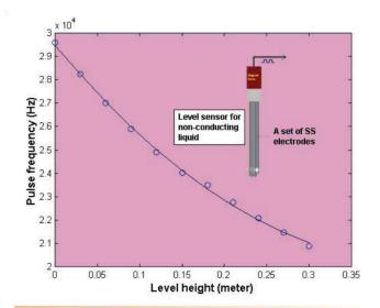
**Fig. 2**Schematic Representation of a Continuous type Pulsating Level Sensor for Non-conducting Liquids and its Response to Level of CCl<sub>4</sub>.
