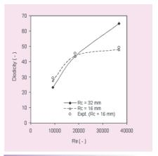
**Fig.8**Variation of Diodicity with Re for Different Radius Curvatures (Rc) of Axial Port Nozzle
