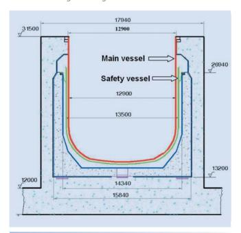
**Fig. 1**Schematic Sketch of Reactor Vault with Vessels
