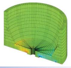
**Fig.6**Stress Distribution in IW Bottom
