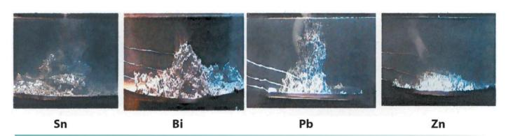
**Fig. 1**Melt profiles for 1 kg Sn, Bi, Pb & Zn Runs in Pool Geometry
