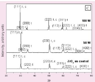
SEM Micrographs of PSZ Coating on type 316L SS, (a) As-coated, (b) Laser Melted at 100 W, and (c) XRD pattern of Laser Melted Samples.
