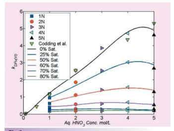
**Fig.3**Variation of Pu(VI) Distribution Coefficients with Aqueous Acidity in PUREX Process. Experimental Data for 1-5 N Acidity was generated at BARC.
