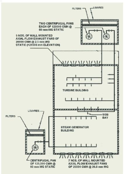
**Fig. 1**Simplified Schematic of Augmentation of Ventilation for Steam Generator and Turbine Buildings
