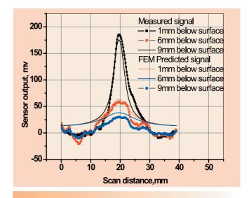
**Fig.3**FEM Simulated and Experimentally Measured Response of GMR Sensor for Sub-surface Notches in Carbon Steel Plate.
