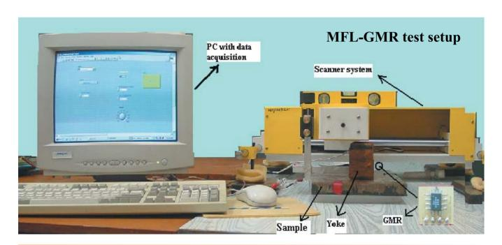
**Fig.1.**MFL Test Setup Comprising of Computer Controlled Scanner for Scanning Surface of the Material with Magnetic Yoke and Sensor Setup.
