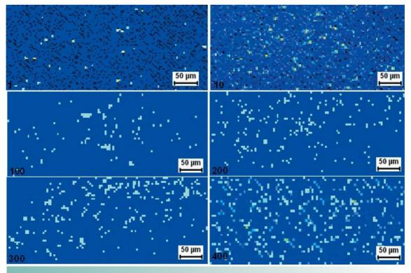
**Fig.2**SIMS Results Showing P-segregation at Prior Austenitic Grain Boundaries of 0% CW Mod.9Cr-1Mo Steel
