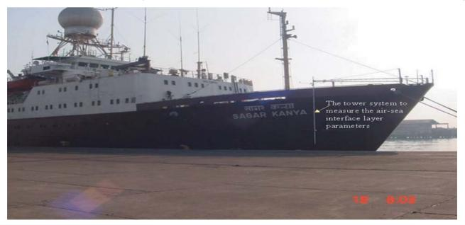
**Fig.1** The ORV Sagar Kanya and the IGCAR Meteorological Mast
