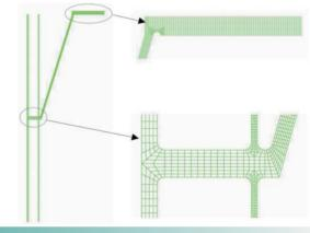
**Fig.2**FE model using 8 noded Axisymmetric Solid Element (QUA8 element)
