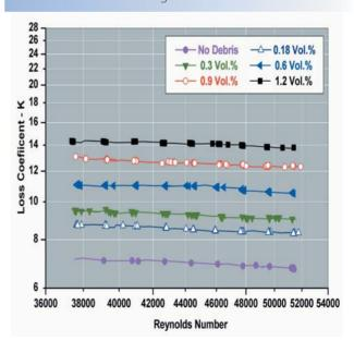
**Fig.6**Variation of Pressure Loss Coefficient with Reynolds Number (for 1.2mm)
