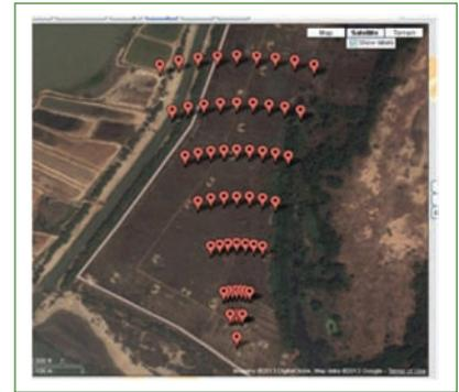
Fig. 2 Layout for aerosol samplers
