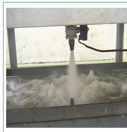
Fig. 2 Solenoid valve with 1 cm² opening
