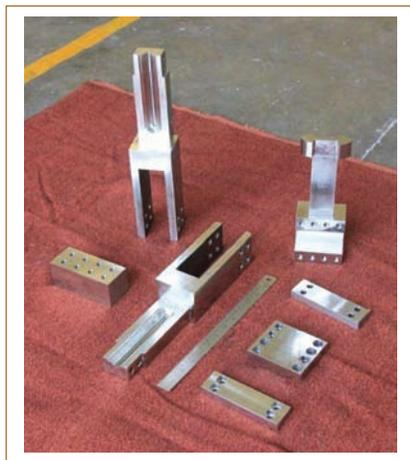
Fig. 2 Machined guide and rails
