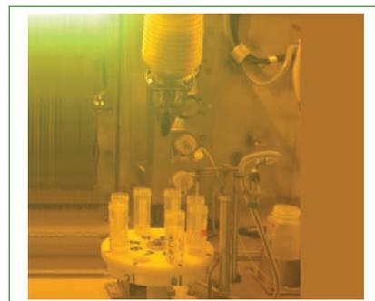
Fig. 2 Sample changer inside radioactive cell
