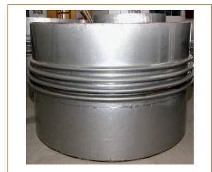
**Fig. 4** Completed bellows
