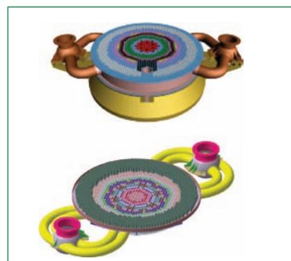
Fig. 3 Bolted grid plate with two primary pipe per header to welded grid plate with four primary pipe per header
