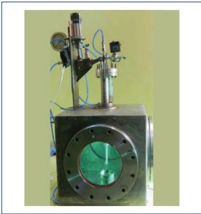
**Fig. 8** Sodium water reaction setup
