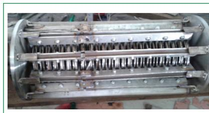
**Fig. 3** Submersible annular linear induction pump with MI cable winding and CRGO laminations
