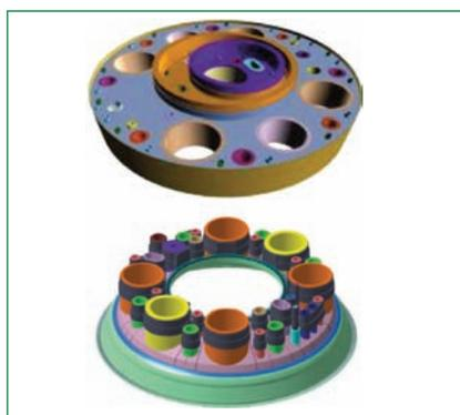
Fig. 2 Box type roof slab in carbon steel to dome shaped roof slab in SS 304L
