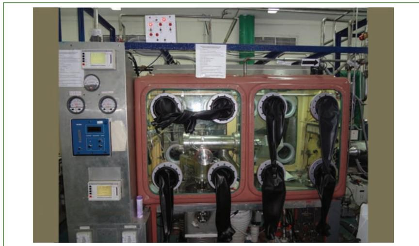
**Fig. 1** High temperature quadrupole mass spectrometer inside glove box
