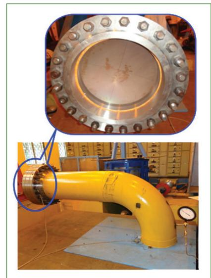
**Fig. 4** Experimental setup for the 20" rupture disc (large size)
