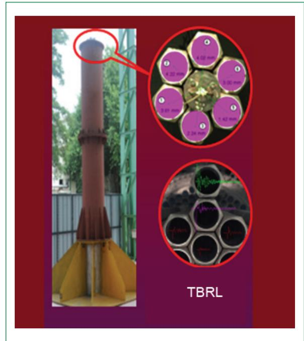
**Fig. 5** Mock-up test carried out TBRL, Chandigarh using low density explosive
