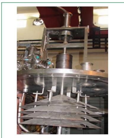
Fig. 3 Top flange assembly showing routing of thermocouples to the IP and internal baffles
