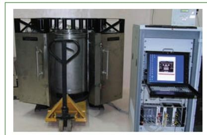
Fig. 1 Photograph of the waste assay system with BF<sub>3</sub> detectors
