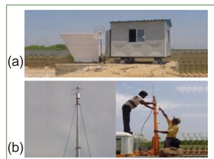
**Fig. 5** (a) Doppler SODAR installed at Edaiyur, IGCAR and (b) sonic anemometer flux measurements
