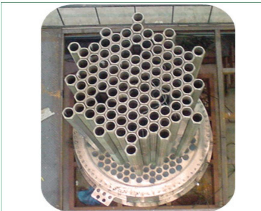
**Fig. 2** Sodium-cooled fast reactor core with subassemblies and grid plate
