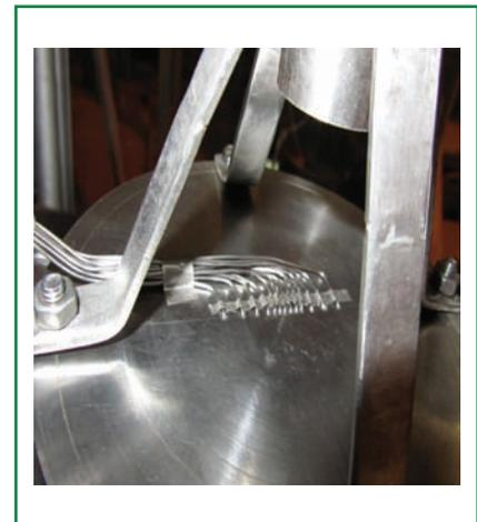
Fig. 2 IP assembly showing the embedded thermocouples
