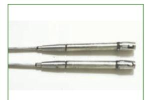
Fig. 3 Laser welded ESPLDs
