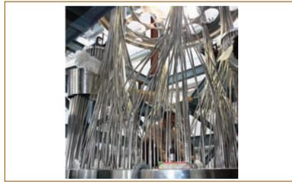
**Fig. 5** Welding of thermocouple tubes
