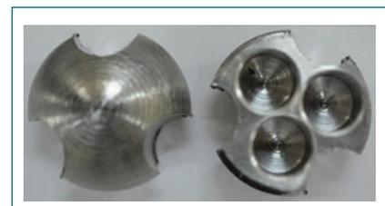
Fig. 2 End plug with slots for sodium flow
