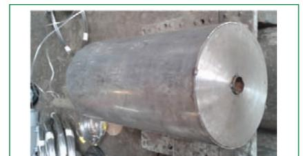
**Fig. 4** Manufactured submersible annular linear induction pump with outer stainless steel cover
