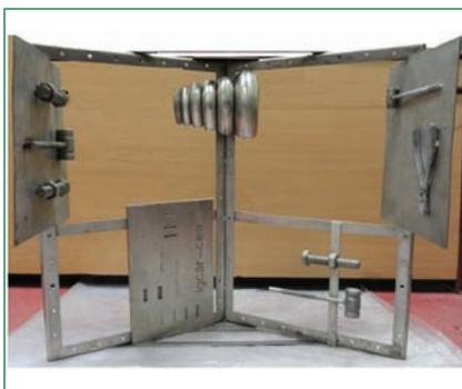
**Fig. 2** Cage structure showing mounting of various tools and objects for under sodium ultrasonic imaging
