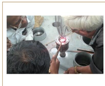
**Fig. 4** Brazing of thermocouples
