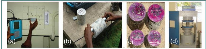
**Fig. 1** (a) Concrete cover thickness evaluation, (b) ultrasonic pulse velocity measurement on core sample, (c) carbonation test for core samples and (d) core sample test
