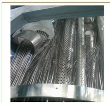
**Fig. 3** View of skirt assembly before shell welding
