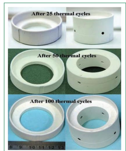
Fig. 2 Photograph of plasma sprayed alumina coated Inconel 600 collars/rings
