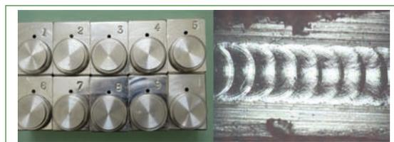
Fig. 2 UT housing welded with crystal mounting caps and the weld profile
