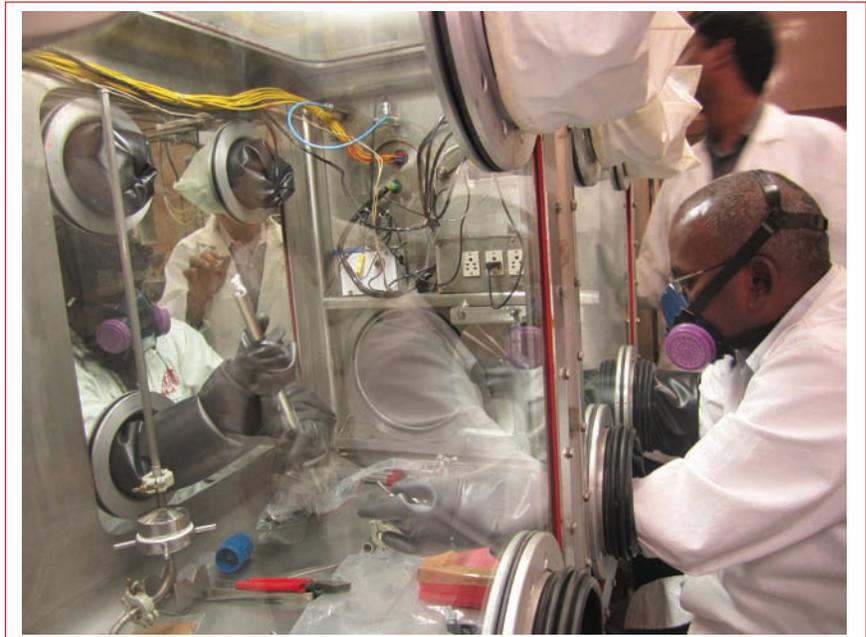
Fig. 1 Metrology and inspection of U-19Pu-6Zr fuel slugs
