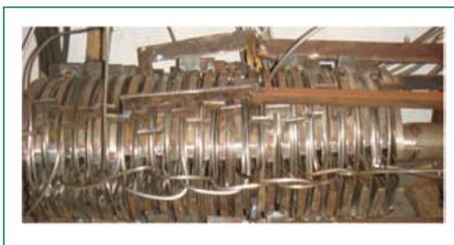
**Fig. 2** MI cable winding of submersible annular linear induction pump along with fixtures and support
