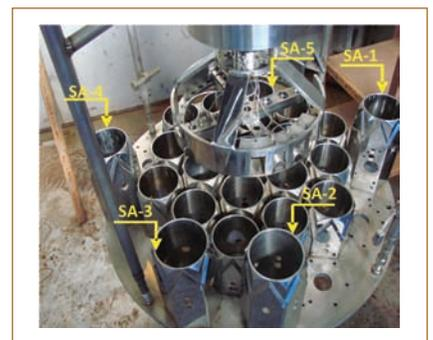
Fig. 2 Target subassemblies and transducer holder with transducers
