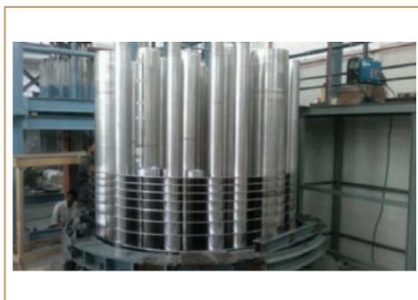
**Fig. 2** Stacking shielding plates in middle assembly
