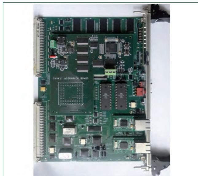
Fig. 2 SHAKTI piggy back board with MC68020 CPU card
