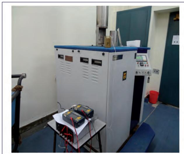
**Fig. 1** Gamma irradiation chamber for testing of electronic components
