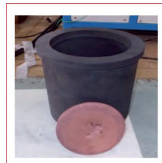
Fig. 4 Copper ingot after melting
