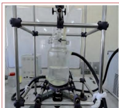
Fig. 1 Constant interfacial area stirred cell
