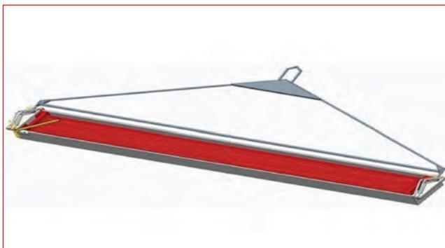
Fig. 1 Proposed setup magazine and magazine holder
