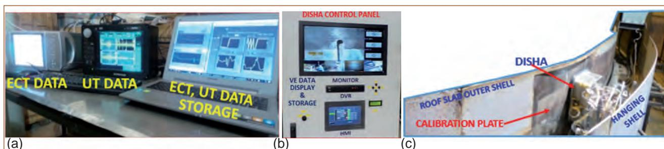
Fig. 2 (a) Ultrasonic test, ECT data acquisition & storage, (b) DISHA control panel and (c) DISHA UT trials on calibration plate in test-rig
