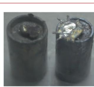
Fig. 5 Liquid cadmium cathode after electrorefining
