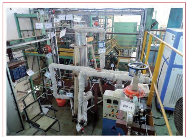
**Fig. 4** Sodium cleaning system setup at Hall 1, FRTG
