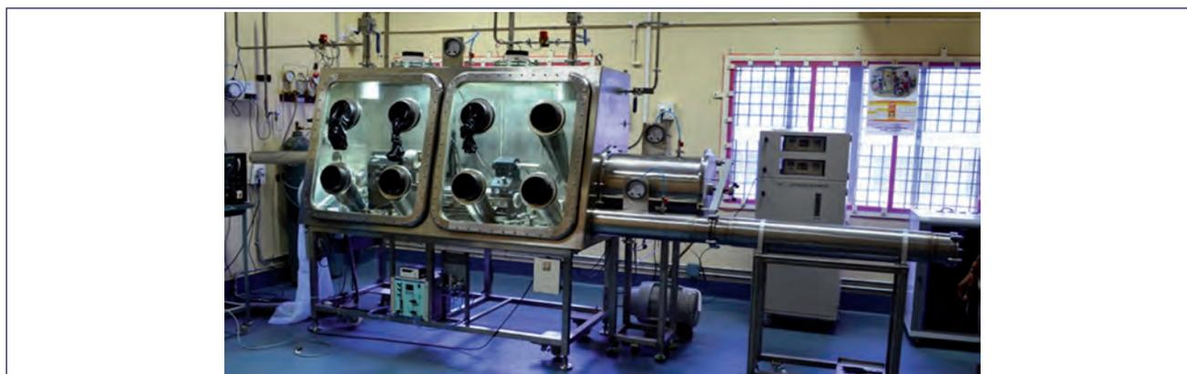
Fig. 1 View of double module SS glove box in ICFF
