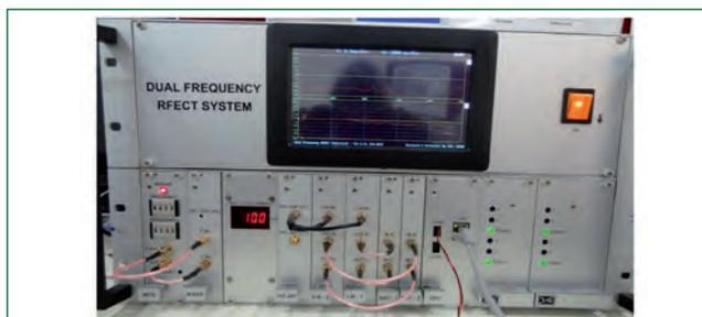
Fig. 1 Indigenous developed RFEC test instrument
