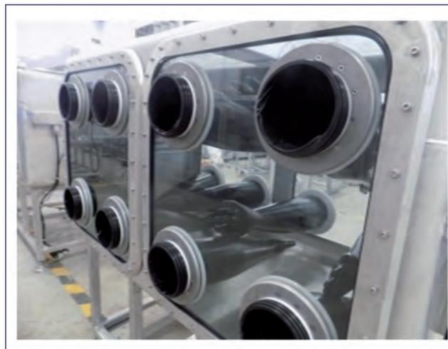
*Fig. 1 Typical glove box*
