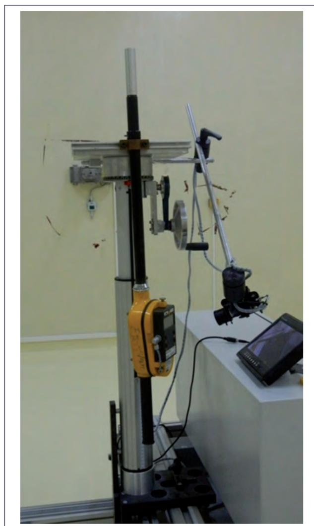
**Fig. 4** Teletector mounted on the calibration table for carrying out calibration, with CCTV camera focusing on the display
