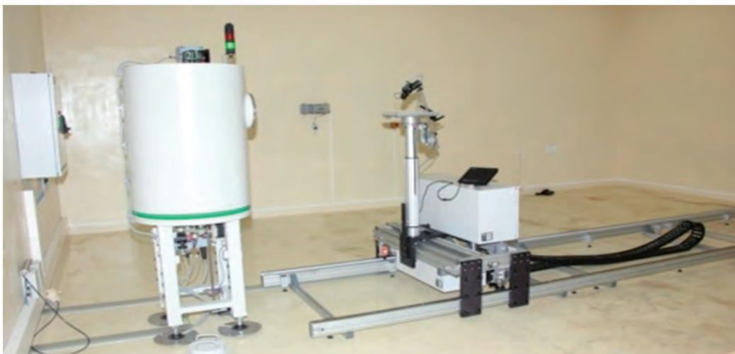
**Fig. 2** Gamma irradiator with linear distancing system
