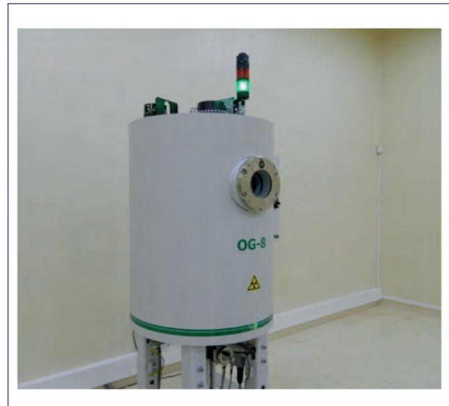
**Fig. 1** Gamma irradiator with six sources
