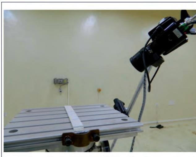
**Fig. 3** Instrument table with CCTV camera for display of instrument readings
