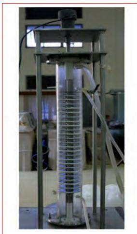
Fig. 1 The experimental setup of ARDC column
