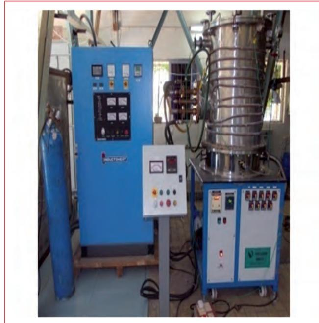
Fig. 1 Induction heating system
