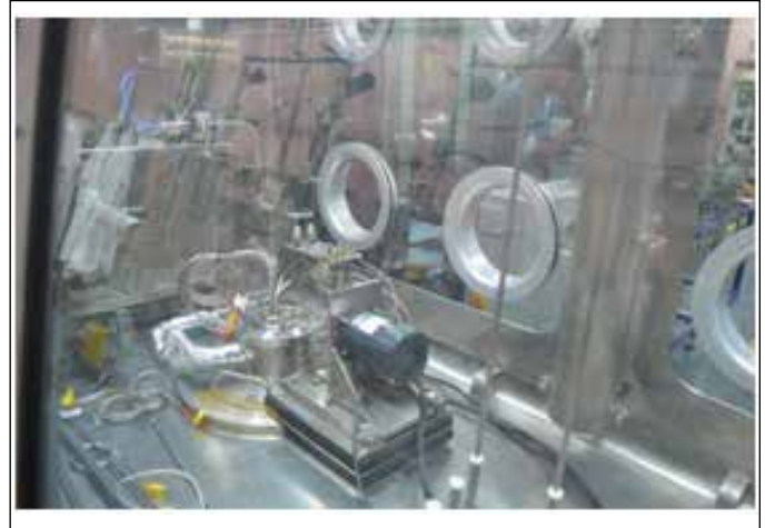
Fig.3: Sodium bonding furnace inside GB
