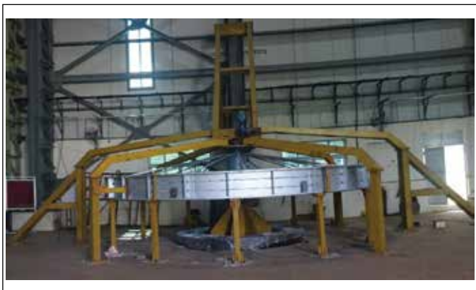
Fig. 1: Large diameter inflatable seal test rig installed in ITSTF
