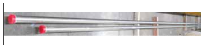
Fig. 3: The first batch of indigenously produced IBR certified IHTA tubes.
