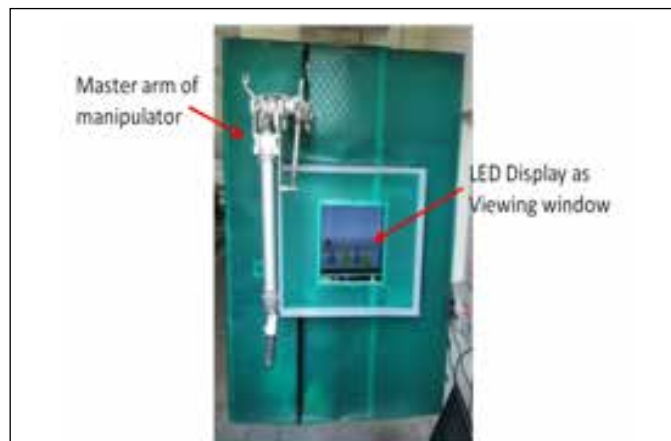
Fig. 2 VR training system for hot cell equipment manipulation
