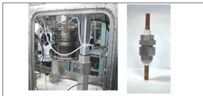
Fig. (2) (a) Vacuum Induction melter commissioned inside glove box. (b) Electrical feed through
