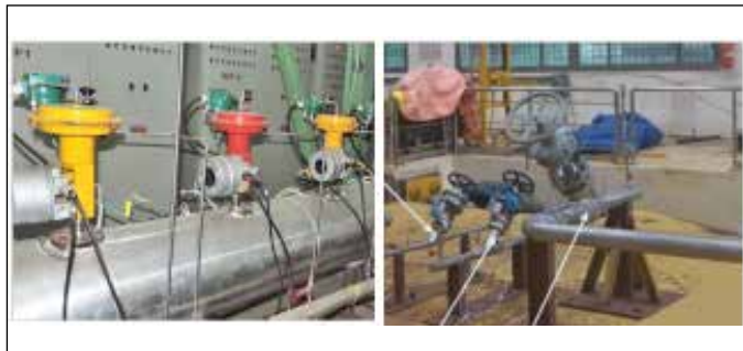
Fig.2 Testing of Inconel 625H bellows in sodium (left) and seismic testing of indigenously developed sodium valves (right)
