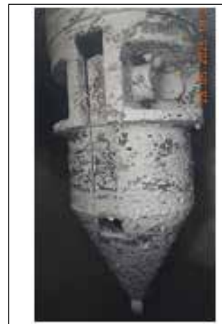
Fig.2 Sodium oxide deposition on the gripper finger region
