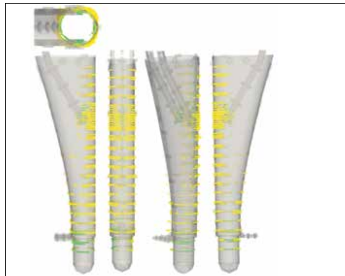
Fig. 2: Visualization of the internals of the spare PTM using the ultrasonic scan data, with corresponding 3D CAD model superimposed for reference
