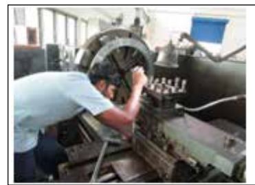
Fig. 4 Machining of Double Dovetail Grooves on Flange
