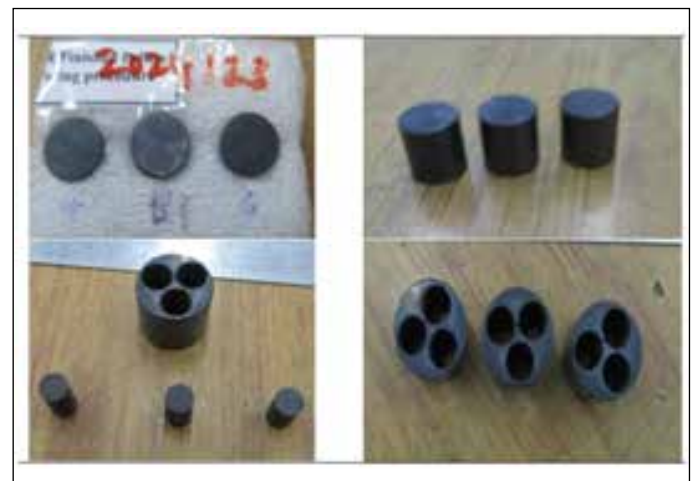
Fig. 2. Enriched boron specimens after machining from the pellets by WEDM sensors.
