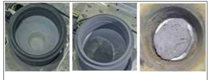
Fig.4 Photos of graphite crucible, collected deposit and consolidated Uranium metal
