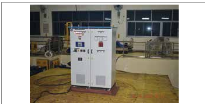
Fig. 1: Prototype 48 V DC charger in shake table
