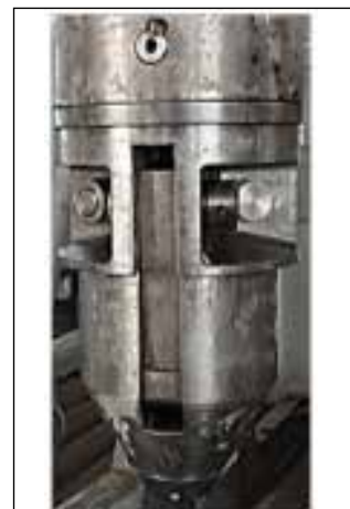
Fig.3 Gripper finger region cleaned using alcohol
