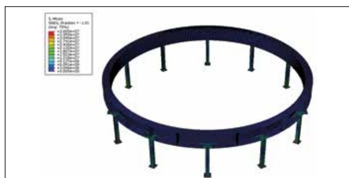
Fig. 4: Von mises stress distribution of outer shell support
