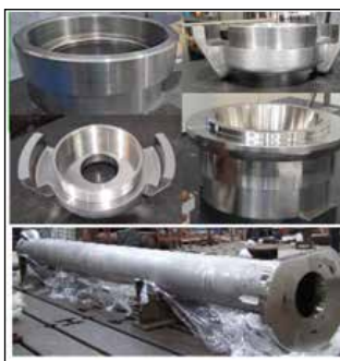
Fig. 7 Hardfaced Parts of Transfer Pot and Final Assembled Transfer Pot
