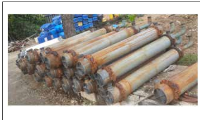
Fig.2: Discarded UF Membranes of Desalination Plant
