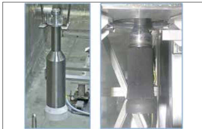
Fig.2 Photos of fresh cathode and cathode with U-deposit
